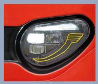
LED headlight has the head light and dipped light functions. The front turn light utilizes the
