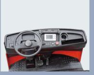
Large screen display, the instrument panel adopts injection molding design, sturdy and
