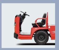
Full suspension operating platform, vibration is reduced, noise is isolated
